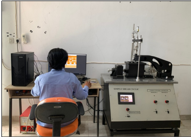
The testing process is carried out using a Simple Shear Cyclic apparatus to evaluate soil behavior under cyclic loading conditions.
